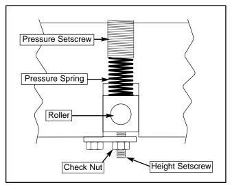
Figure 26. Roller pressure assembly.
